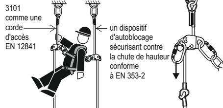
**ASSEMBLAGE DU DISPOSITIF 3101 AVEC LA CENTURIE DE TRAVAIL EN APPUI/CENTURE COAXIALE COMME UN DISPOSITIF DE MAINTIEN EN POSITION LORS DU TRAVAIL ET PROTEGEANT CONTRE LA CHUTE CONFORME A LA NORME EN 358**
